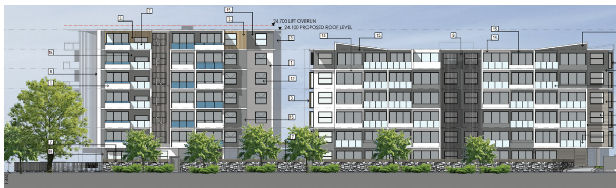
Figure 16: Southern elevation showing lift overrun of Building B (left)
