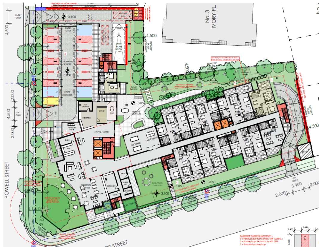
Figure 18: Ground floor plan, amended, showing modulation of the building at this level and its interaction with landscaping
